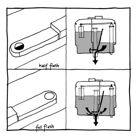
Flushing mechanism for Caroma Dual-Flush toilet
