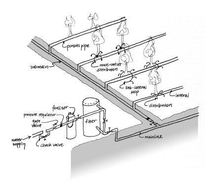
A Typical Drip Irrigation System
