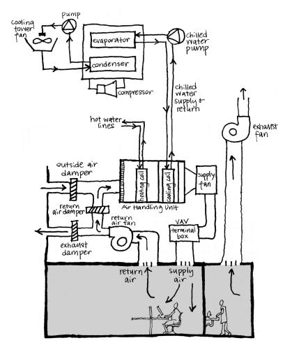
Central HVAC System with Water-Cooled Chiller
