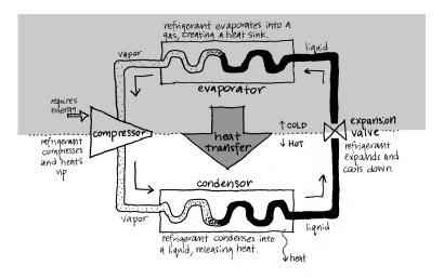
Schematic Diagram Showing Heat Transfer in a Chiller — The Vapor Compression Refrigeration Cycle
